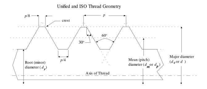
Pitch (p) – The distance between adjacent thread forms measured parallel to the thread axis.
